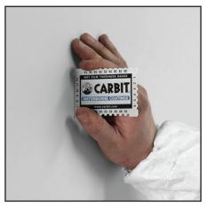
3. Measure wet film to ensure recommended coating thickness for stripping.
